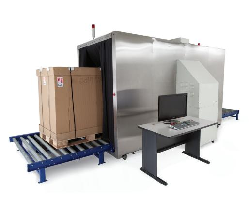
The Autoclear 150180 X-ray inspection system features a large 150.0 x 180.0 cm (59.0 x 70.9 in.) tunnel opening ideal for screening break bulk, cargo, large deliveries and oversized items for weapons, explosives and contraband. The high-capacity system features a low positioned rollerbed for easy pallet loading and offloading for speedy security inspections. Detailed X-ray images with advanced image enhancement tools assist operators to locate areas of concern in densely packed items.
