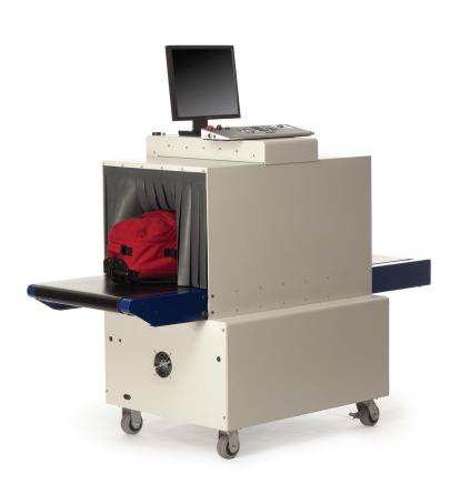
The high-capacity 6848 is designed for inspecting medium-sized baggage, briefcases, parcels and other hand carried items. The unit's 160 kV X-ray generator can penetrate 28 mm (1 in.) of steel, and the L-shaped detector design ensures that objects are scanned in their entirety. The 6848 is equipped with a full suite of intuitive imaging tools that give operators an edge when screening for weapons, explosives or contraband.
