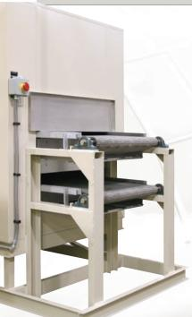
\*Class 100 supply-air out of HEPA filter - Class 1000 workspace environment
