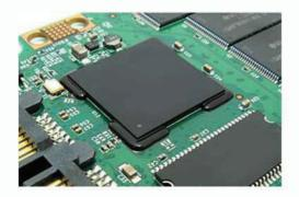
Flip chip underfill curing
